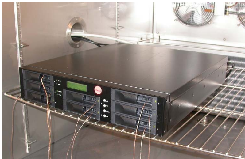
Photo 1 of 4: Chassis in test chamber
